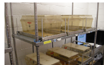
Locomotor behavior chambers used to measure novelty, home-cage, and drug induced locomotion as well as circadian rhythm.
